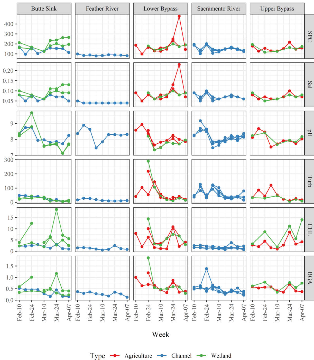
Figure 6. Physical water quality parameter time series at the various cage locations.
